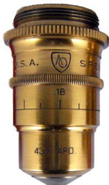
Figure 3. N.A. 0.95 APO Objective with correction collar
