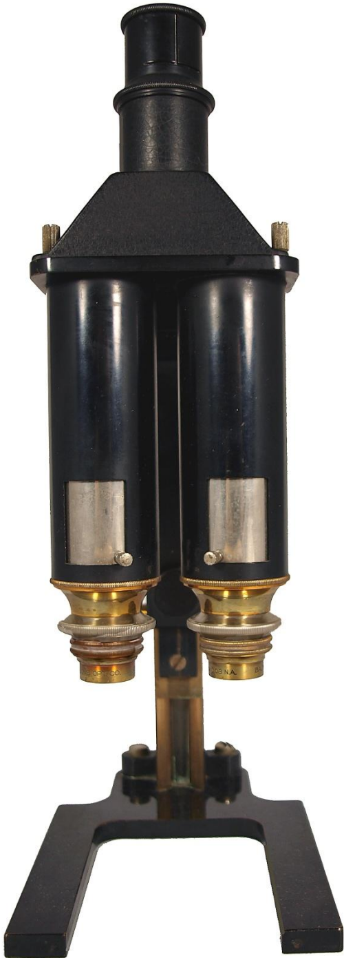
Figure 4. Bausch and Lomb Comparison microscope. c. 1929 front View
