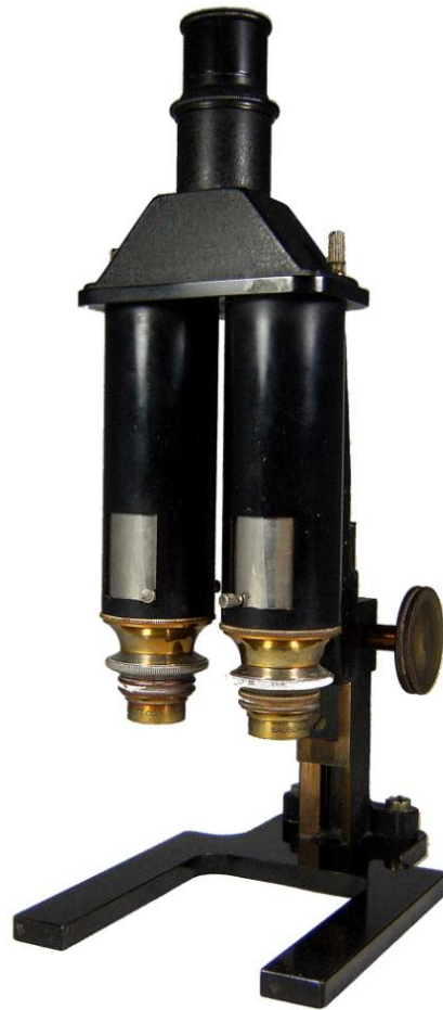
Figure 5. Bausch and Lomb Comparison microscope right-side view
