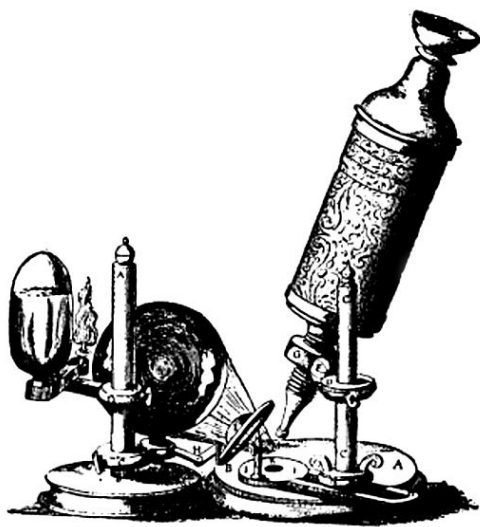
Figure 2. Robert Hooke Microscope c. 1665 used reflected light
