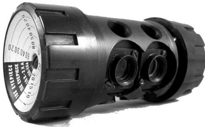
Figure 20. AO Cycloptic® stereo microscope drum, offering five magnifications with two telescopes and "see-thru" openings
