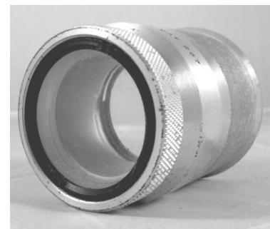
Figure 17. AO Cycloptic "Common Main Objective" with 2/3X No. 267 achromatic aux. lens-attachment
