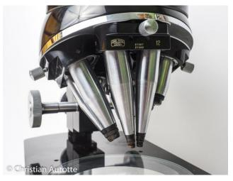
There is some visible wear, some discoloration on the lens turret and on the tip of some lenses. The wooden box is also shows its age, and the door is missing its key. It doesn't have the power supply to light the lamp that sits in the middle of the lenses, but there is a mirror if one needs to light a subject from below. There is no way to move a slide mounted subject, but that was not meant to be, as we will see shortly.
