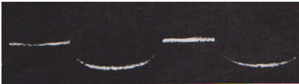
Fig.7 Stereo (printing block) depth of etching: 59 \mu\text{m}
