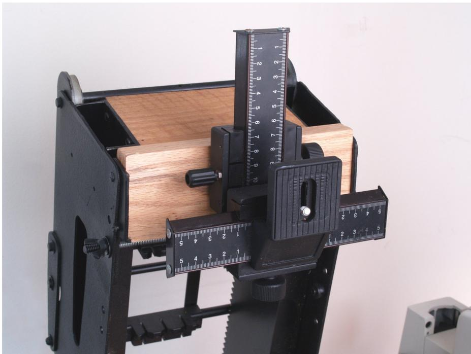
The focusing rail was necessary to be able to align the camera with the microscope for parfocality.
