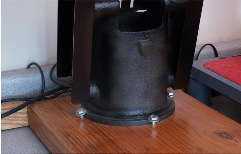
The top of the enlarger column was closed with a block of oak and a focusing rail was mounted on another block of oak to accommodate the camera. The flanges on the sides of the column were squeezed in to lock them in place with a 1/2-20 threaded rod, as can be seen just below the oak block holding the focusing rail.
