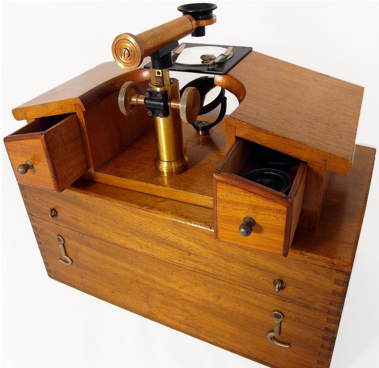
Figure 23 . Verick - Simple dissecting microscope on its relatively large stand
