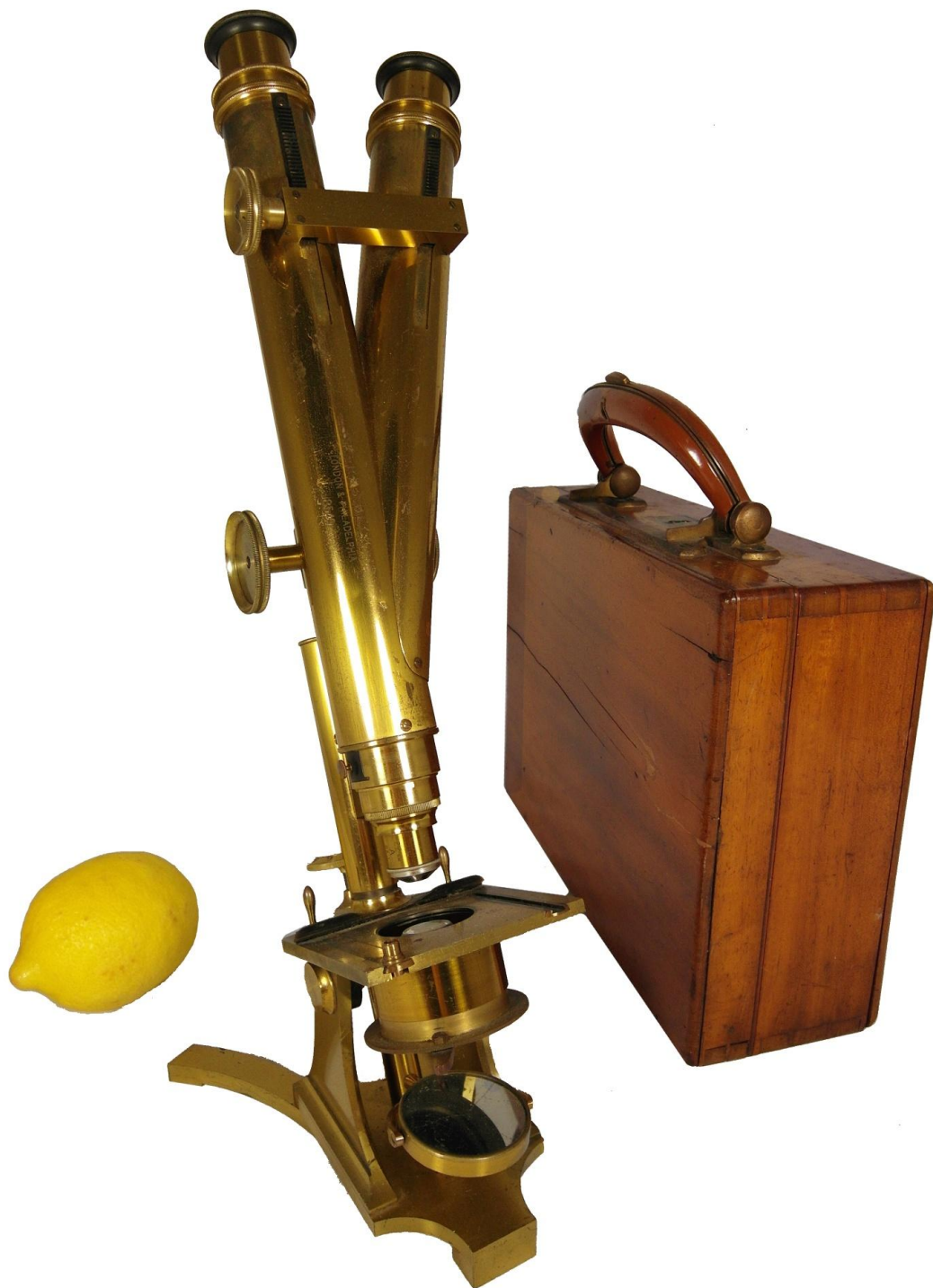
Figure 35. Beck field portable Wenham stereo binocular with its unusual travel case
