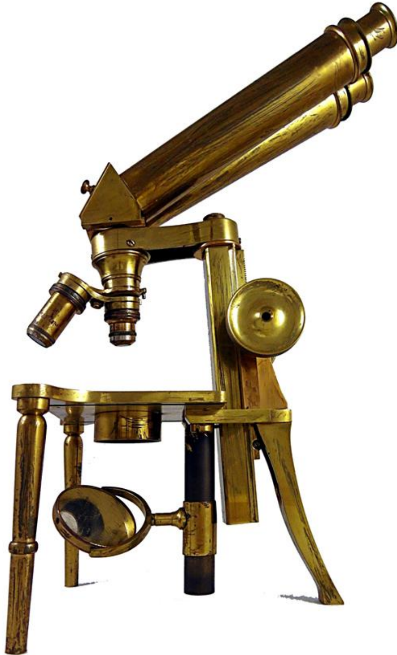
Figure 31. Riddell-Stephenson style stereomicroscope made by J. Swift and Son
