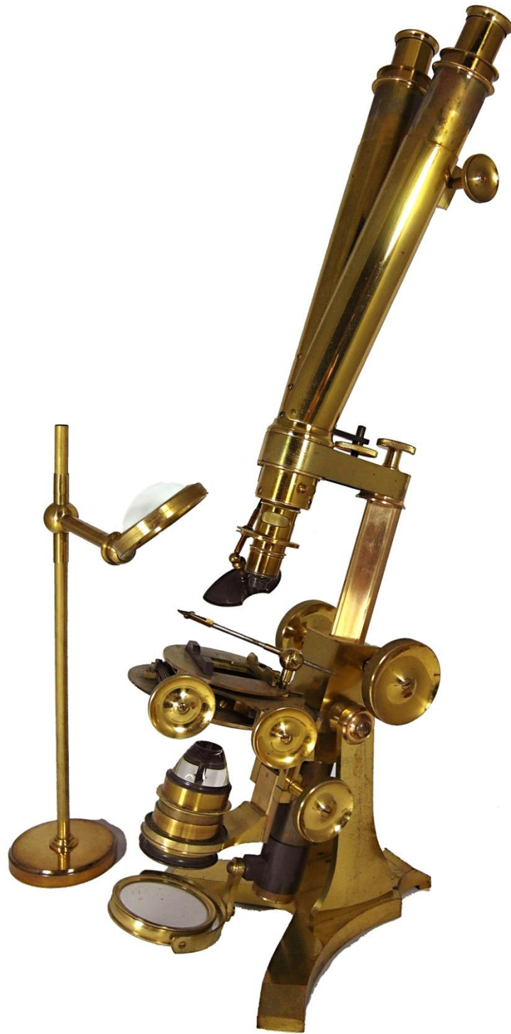
Figure 36. J. Swift large Wenham stereo binocular, over 23 inches tall as shown
