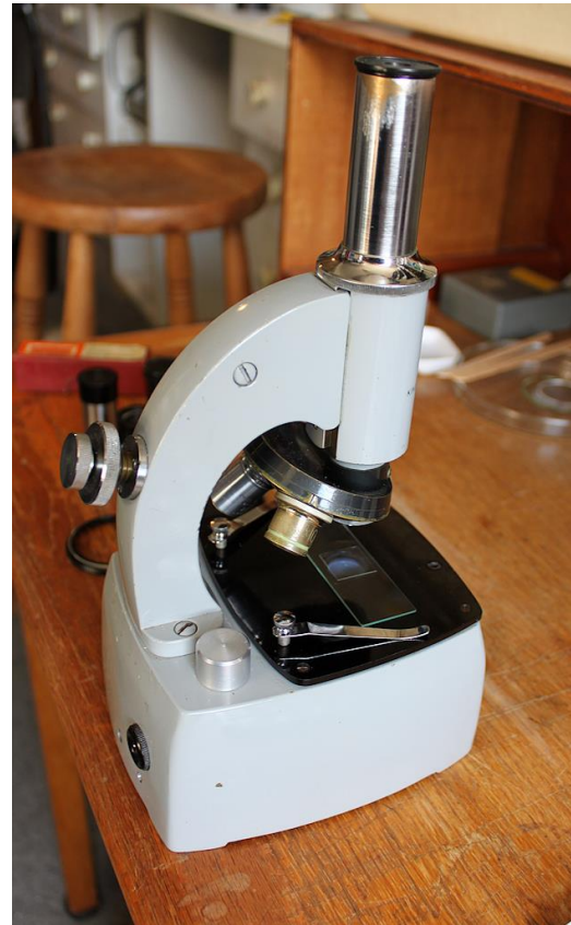
The Prior school microscope – newer model New brightness control knob on top
