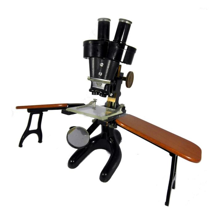
Figure 4. Bausch and Lomb Greenough Stereomicroscope, ca. 1929, Rochester, USA.
