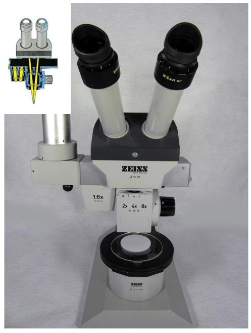
Figure 7. Zeiss Stemi DRC Greenough-style Body with Photo Port and Equipped with Changer D 2x-4x-8x, the 1.6x Objective Pair, and Transmitted-light Bright and Dark Field Illuminator, on an LO Stand, 1978.
