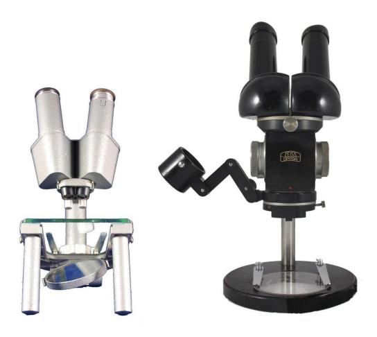
Figure 9. Leitz Greenough Side-by-Side with Zeiss Opton CMO Stereomicroscope, 1949, Inclusive 6x-10x-16x-25x-40x Magnification Changer like Zeiss Jena Citoplast, 1946.
