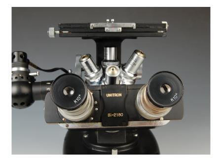
The binocular head can be adjusted to interpupillary distance by rotating the knurled collar on the left eyepiece tube. Rotation of the diopter collar on the right eyepiece tube allows compensation of differences in vision between the two eyes.
