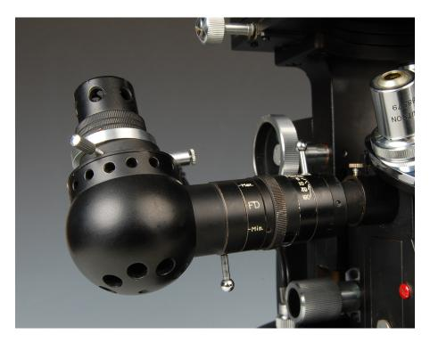
The illuminator uses a very weak 8 volt, 12 watt EL-2 bulb. The lamp house has centering screws to align the lamp filament with the condenser. The condenser has a Field Diaphragm and an Aperture Diaphragm. The opening travel on the Field Diaphragm is very generous, whereas the travel on the Aperture Diaphragm starts at small and goes to smaller. So, if one expects to enhance contrast and depth-of-field by stopping down the Aperture Diaphragm with a 12watt lamp, the resultant image is very murky.
