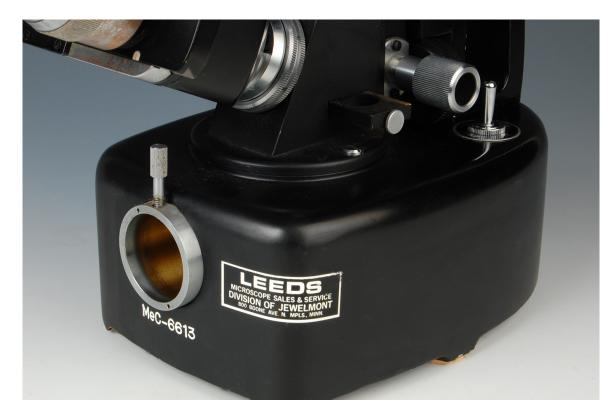
The port could accept the accessory TYPE MC-M35 35mm camera back or a Polaroid camera for instant photography. I was not able to track down either of these cameras. Just below the fine focus knob on the left side is a "slideway" that allows images to be directed to either the viewing head or the camera port. Moving the slideway to the right sends the image to the viewing head and sliding it to the left sends the image to the camera port.
