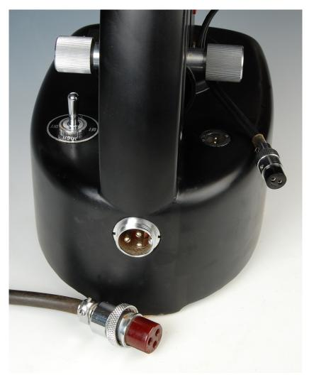
The 120 VAC cord plugs into the rear base of the microscope. The voltage to the illuminator is controlled by the ON/OFF/HIGH/LOW selector toggle switch. The third lead is grounded to the microscope chassis. The illuminator uses a two-pronged plug.
