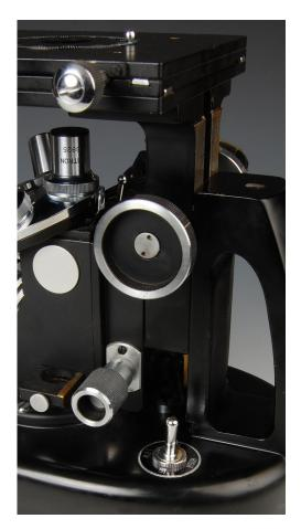
There are knobs for coarse and fine focus on both sides of the microscope. The drag on the coarse focus (the stage) can be adjusted by gripping both coarse focus knobs and turning them against each other to the desired tension.
