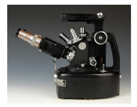
The microscope has a four position objective turret. The set came with 5X, 10X, 20X, 40X and 100X Oil objectives.
