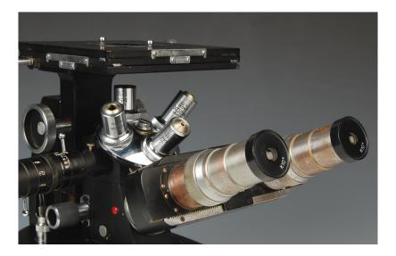
Immediately below the turret is the "PLANE GLASS REFLECTOR" lever, which is the beam splitter for epi-illumination. The beam splitter in my sample was so far gone, I replaced it with a glass coverslip. By eyeballing the illumination as the lever is rotated, one can find optimum illumination. However, rotating this lever requires imaginative maneuvers with hand tools.
