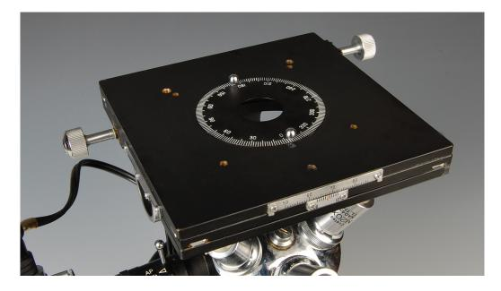
The stage plates have beveled edges so they simply drop in. The stage is also threaded to accept stage clips. The X-Y movements of the stage can accommodate gross specimens.
