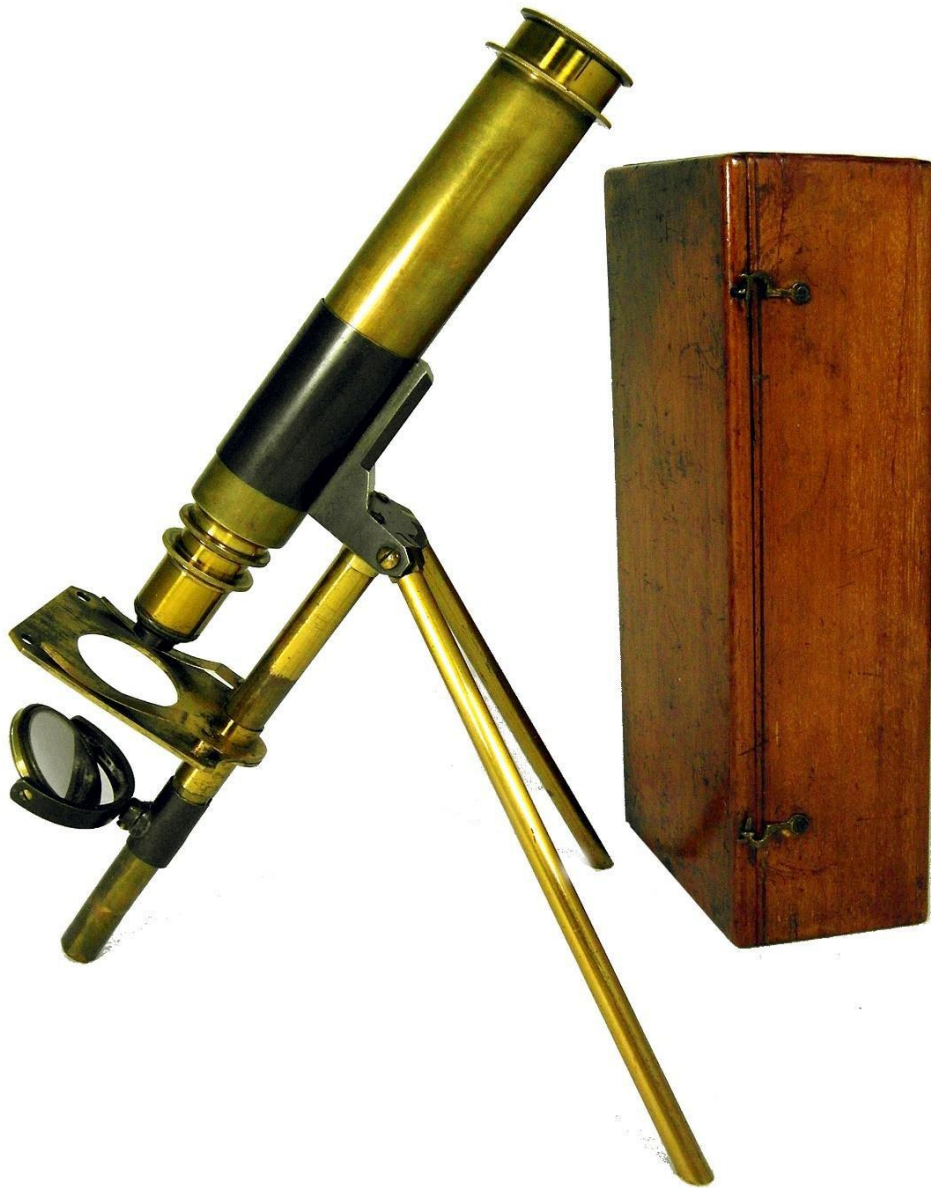
Figure 22. Moginie-style microscope by unsigned manufacturer with unsigned objective (likely 1" by Couch)
