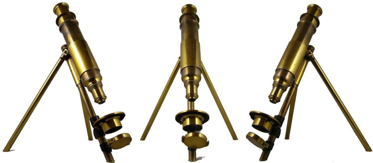
Figure 2. Baker's Original Moginie-Style Field Microscope
