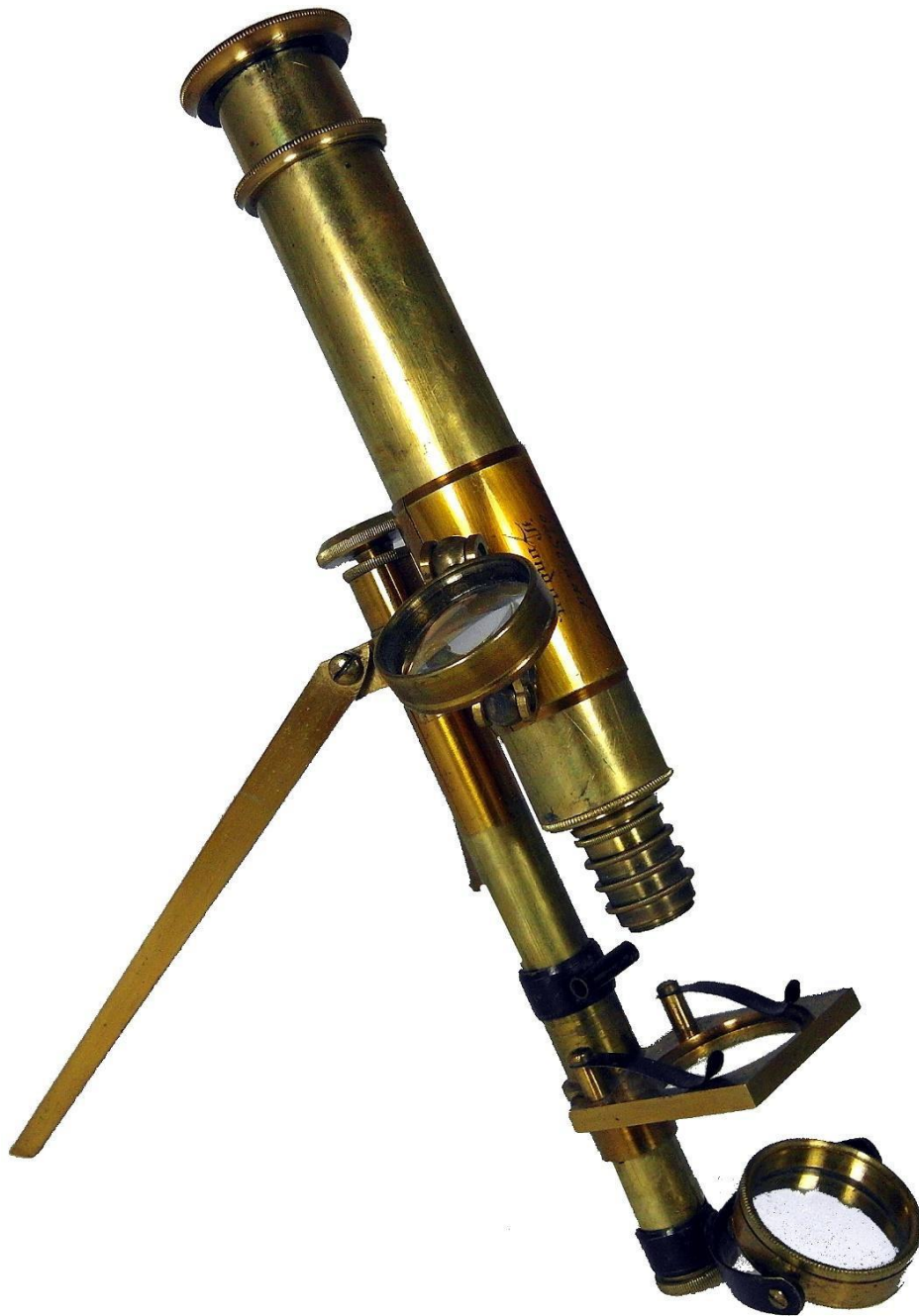
Figure 20. Browning microscope, about 8-1/2" tall, as shown, 12.4
