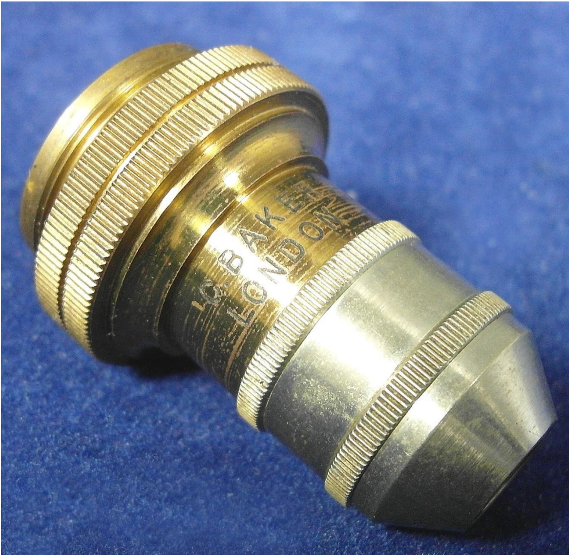
Figure 12. 1/2 Inch C. Baker Objective
