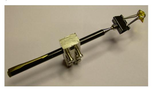
Now you can see why the Bulldog clip had to be of this type. There is sufficient spring in the wires in this position to hold all sorts of interesting items for the stereo microscope and the large brass block is quite stable but can be clamped through it's mounting holes or just held using some double sided tape or BluTac.
