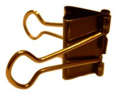
Now I needed a method of holding the clip, I decided to drill through the spring steel! This was a mistake as my mini drill with a 1.5mm tungsten carbide bit would only scratch the surface, but did go over 12mm into my left thumb very easily when it slipped. Anyway, once the bleeding had stopped, I attacked the clip with small diamond grinding attachments and successfully made a hole for a 3mm screw.
