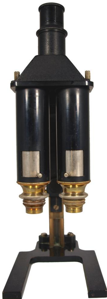
Figure 4. Bausch and Lomb Comparison microscope. c. 1929 front View
