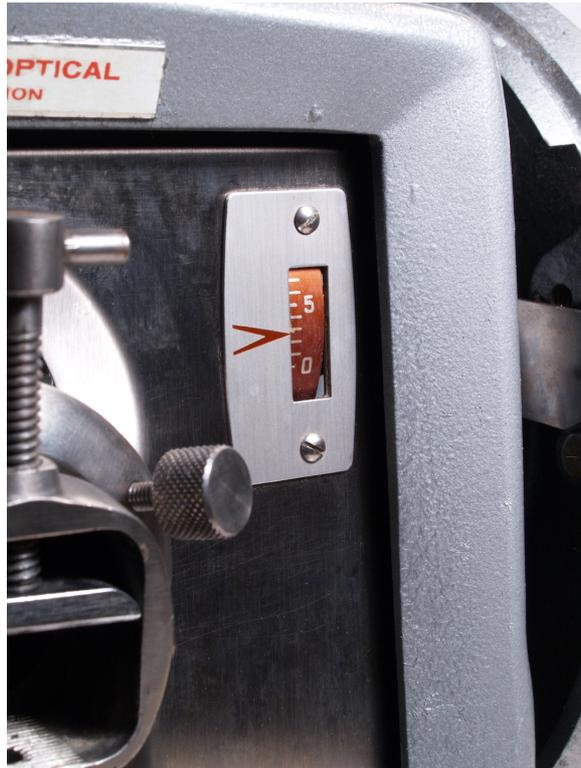
The mounted paraffin block is clamped into the object clamp which is secured into the drive mechanism with three knurled screws.
