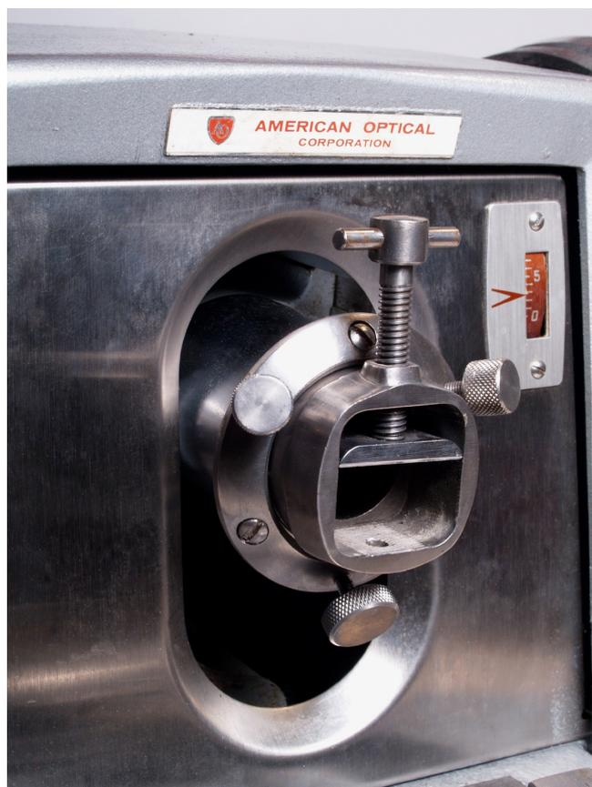
locked into position. Drawing the locking lever will unlock the drive wheel so sectioning can begin.
