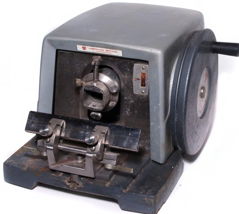
And here it is after de-rusting, buffing with wire brushes with a Dremel motor tool, buffing with steel wool and repainting.
