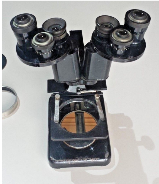
Leitz stereo microscope ca. 1920s. Image by the German eBay seller 'tug2003'.
