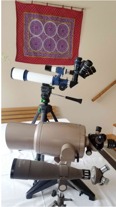
Left. Three telescopes with multiple eyepiece turrets. Centre. 70mm Eschenbach refractor with a four-eyepiece turret. Right. Baader four position eyepiece turret onto a 60mm Carton refractor.
