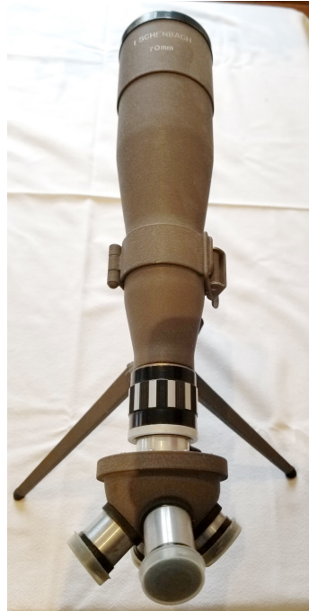
Left. Three telescopes with multiple eyepiece turrets. Centre. 70mm Eschenbach refractor with a four-eyepiece turret. Right. Baader four position eyepiece turret onto a 60mm Carton refractor.
