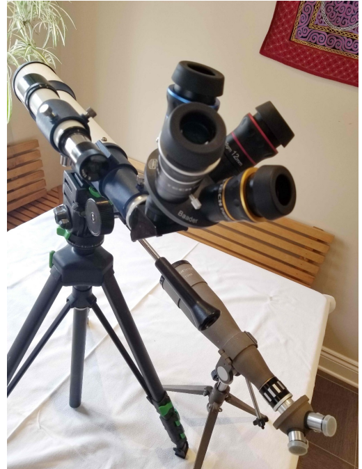
Left. Three telescopes with multiple eyepiece turrets. Centre. 70mm Eschenbach refractor with a four-eyepiece turret. Right. Baader four position eyepiece turret onto a 60mm Carton refractor.
