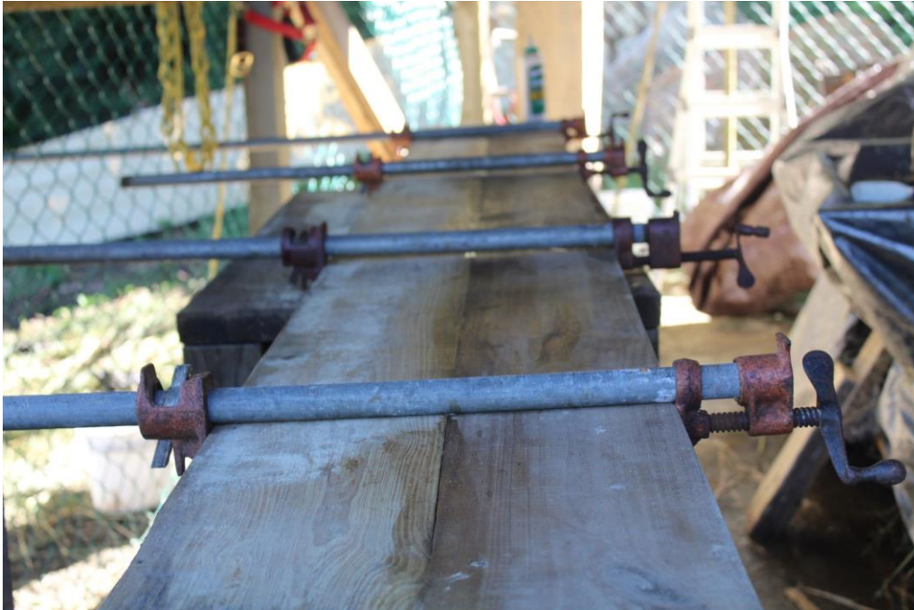
Half of Benchtop being glued. Glue time is a whole 24 hours or more depending on humidity
