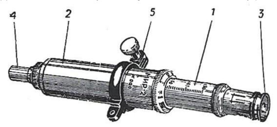
thereby changing the increase in magnification. Increase with tube length 130 mm - 19X, with a tube length of 160 mm - 26X, with a tube length of 190 mm - 33X.
