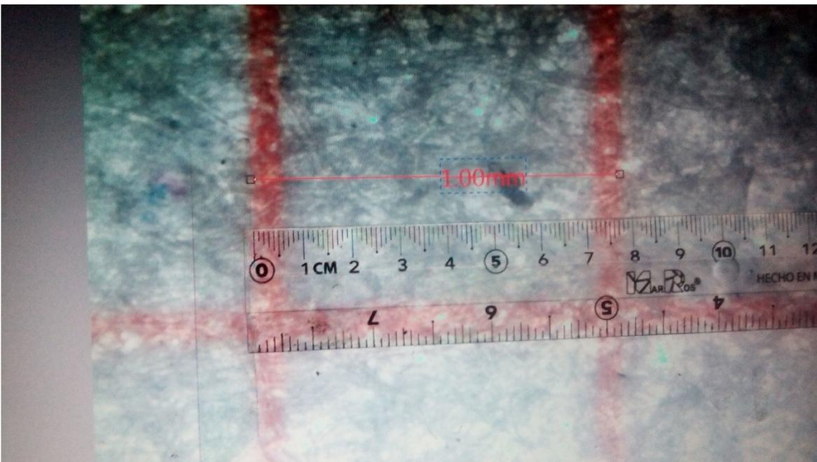
With a conventional ruler I measure that length that it is going to be the reference value: **1 mm is 7.8cm at 20% zoom** in this software and on this computer.
