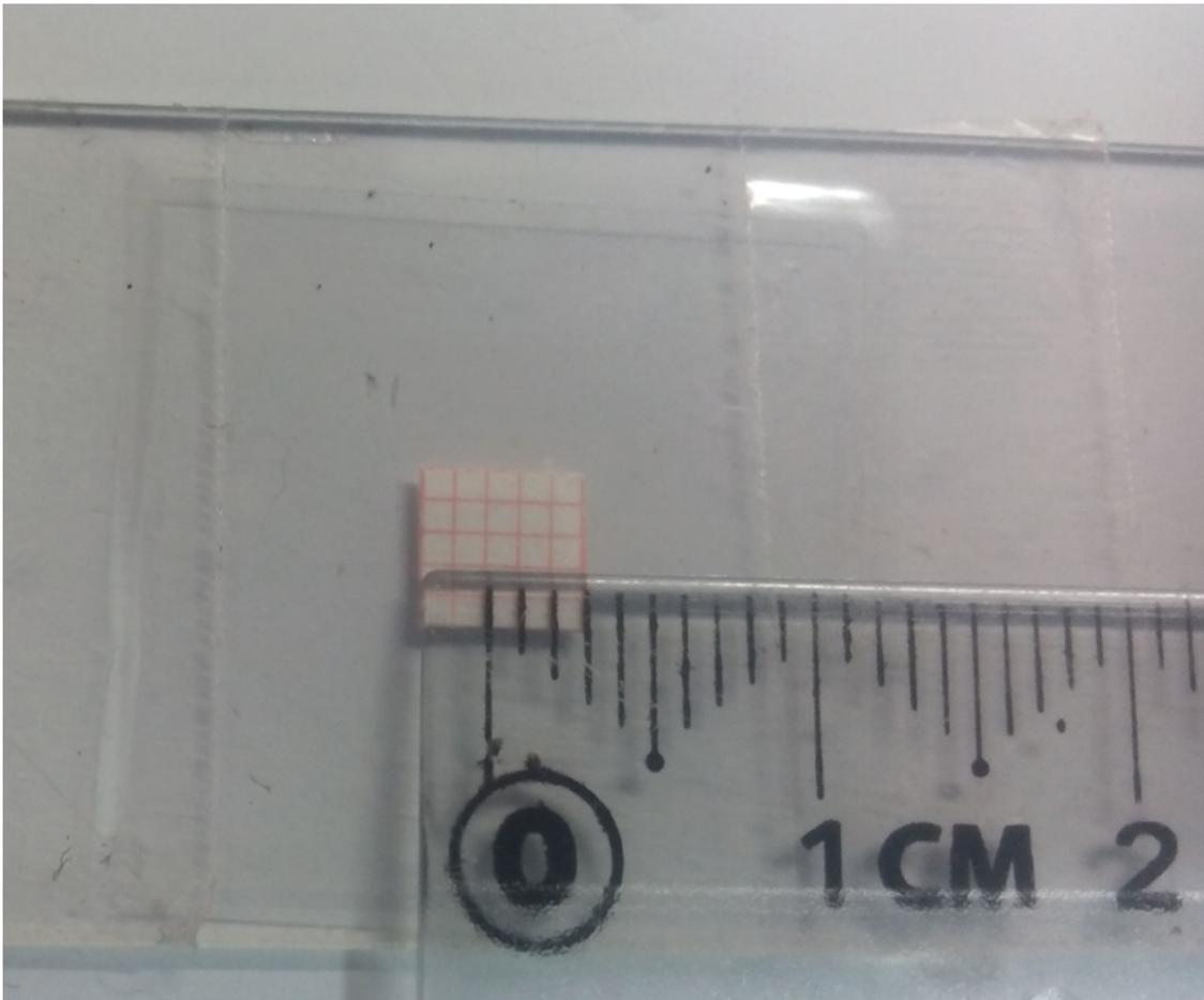
With the 4x objective on the microscope I open the software of my camera and measured the length of one millimeter in my computer at 20% zoom. Since my camera is already calibrated and with the purpose of showing the accuracy of this method, I demonstrate by measuring with the same camera that the square is one millimeter across.
