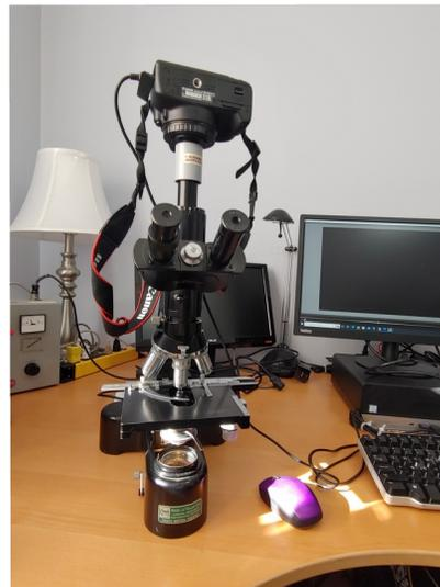
It is possible to install the adapter directly in the trinocular port and obtain an image from only the objective lens. This method produces a less than ideal image quality for a variety of reasons. To achieve a higher quality image, I have utilized a Leitz trinocular port to 23.2 mm adapter, a 10X ocular lens and a modified pvc plumbing fixture with one end providing a snug fit around the ocular lens housing and the other end with a 23.2 mm diameter to receive the camera to microscope adapter.
