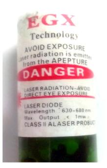
In my case since a wide range is given for the wavelength of the laser beam, I am going to take for granted the common data as an average of 650nm for the moment. But at the end of this paper I am going to demonstrate how to calculate more accurately the wavelength of my laser pointer and how an accurate value of the wavelength can give a better result.
