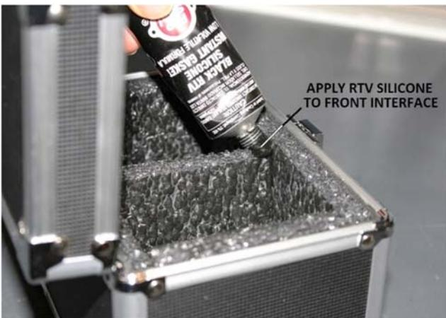
Use your finger to evenly spread the RTV silicone and to remove any excess.
