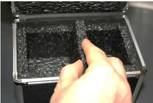
Carefully apply silicone RTV to the vertical interface where the center divider contacts the top of the front foam piece.
