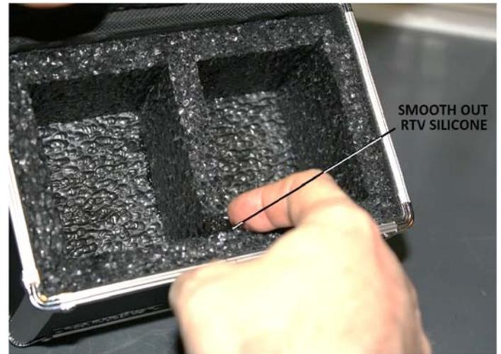
Carefully apply silicone RTV to the vertical interface where the center divider contacts the top of the rear foam piece.
