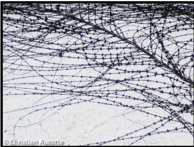
Mounted too quickly and carelessly, this slide shows a lot of dirt. A dip in acetone and more care in cleaning the slide could have prevented that.
