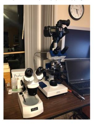
The scope has three lenses in a closed turret with 1x, 2x, 3x or with 2x, 3x, 4x objectives. The eyepieces are advertised as WF 10x, but the oculars I got were 20x so I emailed and asked for replacements. They responded in less than an hour, said they'd ship the 10X, and "Please keep the 20x". How's that for customer service! Note: they're 30.5mm lenses, so you can't use old 23.2 oculars if you have some laying around.
