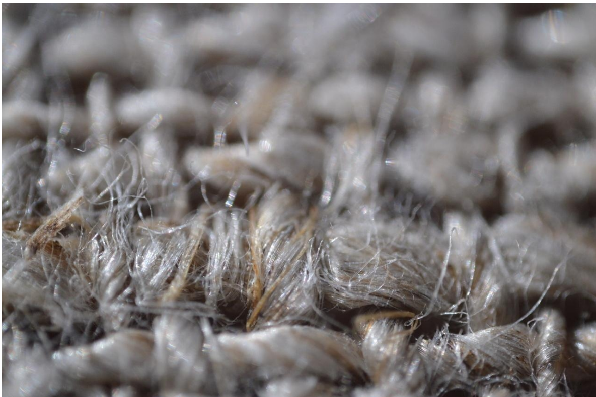
Fabrics above with 120mm tube in APS-C camera and 3.7-0.11 LOMO. You need several shoots and a focus stacking program to generate more sharpness. Width of the picture is about 7 mm.
