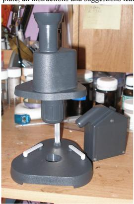
The light source is a simple battery powered tungsten torch which provides adequate lighting for the x20 magnification (and "ok" lighting in a pinch when travelling, for the lower magnifications of a "freshman" microscope as described in Grays "basic micro technique") being battery powered it ideal for travelling with the 'scope.
