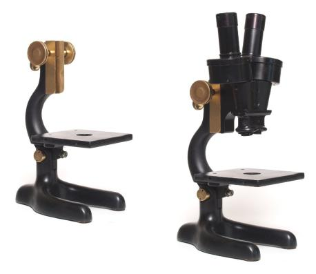
The stage appears to be bronze and was stripped of the original paint. Neatly engraved on the stage was an item number VN-95835AT. On top of the left erecting prism housing is engraved "BAUSCH & LOMB OPTICAL CO. Rochester N.Y. U.S.A 178855".
