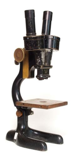
When first trying it out, I couldn't get sharp focus in stereo. I replaced the eyepieces with a matched pair of 15X eyepieces and still could not get focus in both eyes simultaneously. I emailed Jordan and asked him if he had any ideas, and he responded that the scope may have been out of collimation due to an impact. On closer examination I discovered two things:
