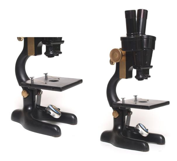
All I had to do was fabricate the swing arm for the substage mirror assembly and add felt pads for the foot and the restoration was complete.
