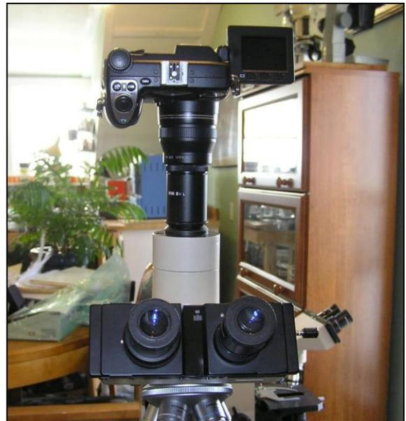
Figure 5 shows the Nikon CP5000 mounted on a BH2 with its 8x eyepiece and adapter, and view screen rotated. Not many controls are easily accessed (the ones on the camera top). In addition, you might want Nikon accessories such as power adapter, wired remote control, and USB computer cable. These are all available on eBay.
