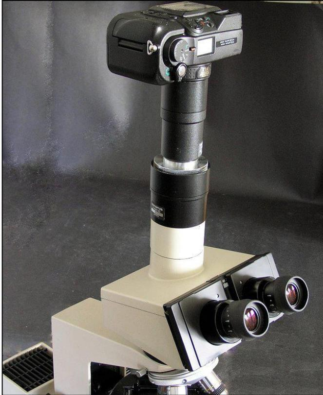
Figure 11 (left). Mounted neatly on a BH2 trinocular head, this C-4040 with adapters C3040-ADL and U-PMTVC provide excellent digital images.
