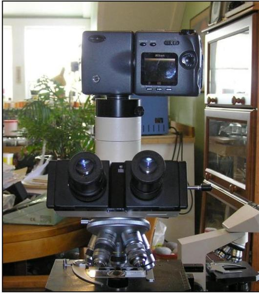
Figure 3. CP990 with a Zarf adapter, also housing a Zeiss 8x relay eyepiece.
