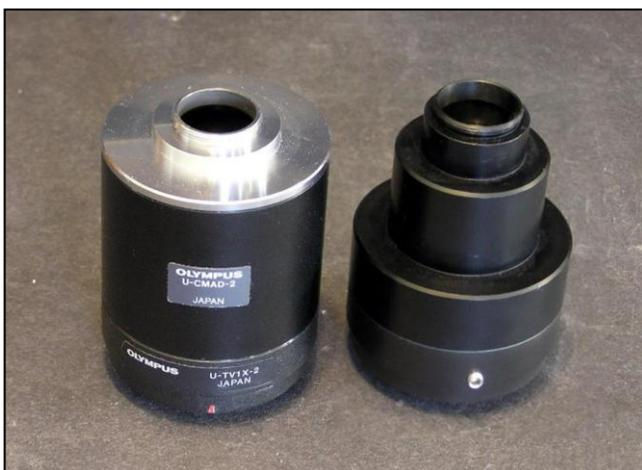
Figure 10. U-CMAD-2 and U-CMAD-3 c-mount connection tubes for BX heads.
