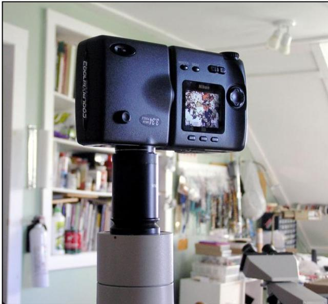
Figure 2. Nikon Coolpix 995 and Olympus 8x eyepiece adapter.
