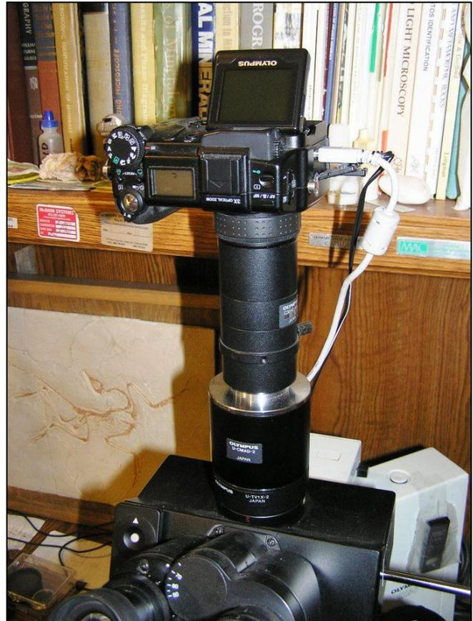
I like the C-5050 camera as it feels very solid and well designed. Olympus did a good job with making it work well on the microscope via the special adapter tube. The cameras are cheap enough now but the adapters are usually expensive, although once in a while a bargain appears on eBay.
