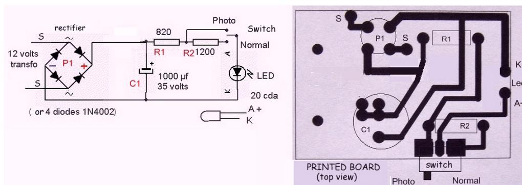
Voltage from the transformer (12 volts) is applied to the rectifier P1 then smoothed by capacitor C1 (\*see Note 1 ); 12 volts AC becomes 19 volts DC.
