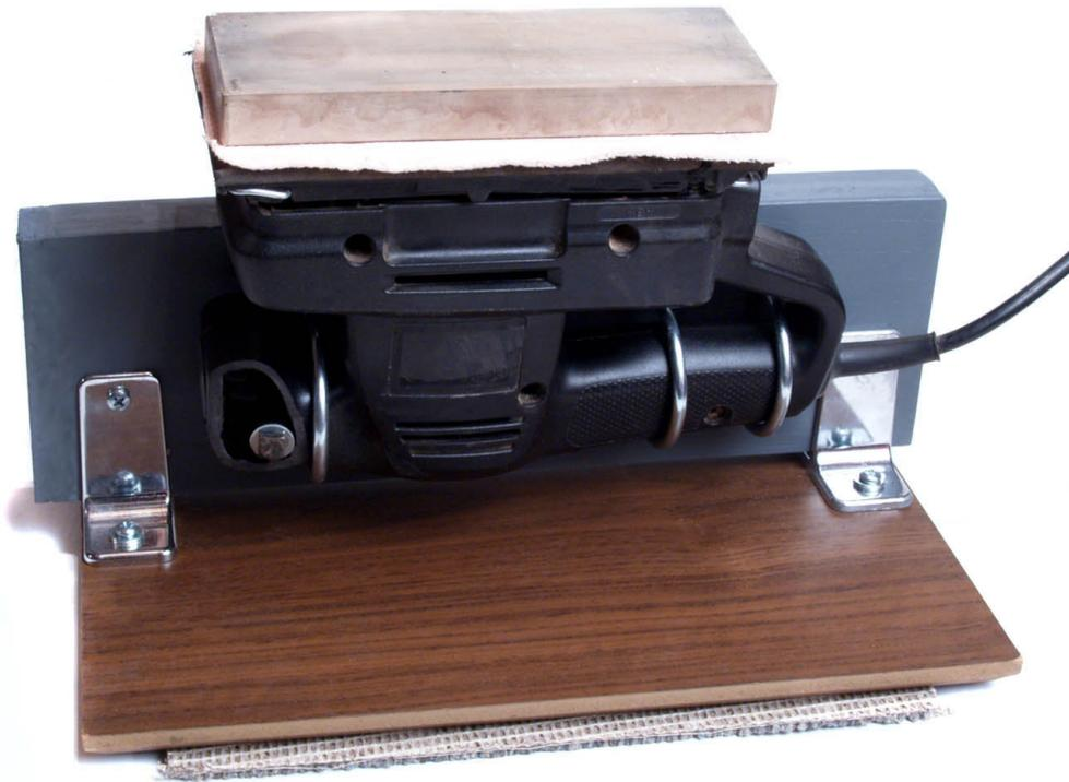
The sharpener needs to be clamped to the workbench using C-clamps to keep it from creeping around. I hold the knife to be sharpened with a vise-grip and let it rest on the stone under its own weight. After sharpening with water I can then go to the fine and then the finest grade of diamond paste.
