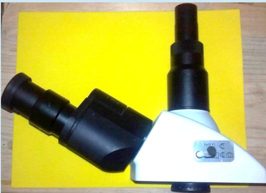
I removed the trinocular head and placed the filter on the base of its lowest optical element.
