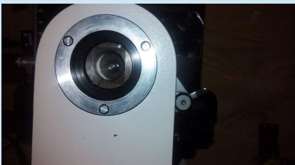
The other method that I used was to place the analyzer filter directly upon the sample and the polarizer for both methods upon the illuminator. Both methods performed very well.
