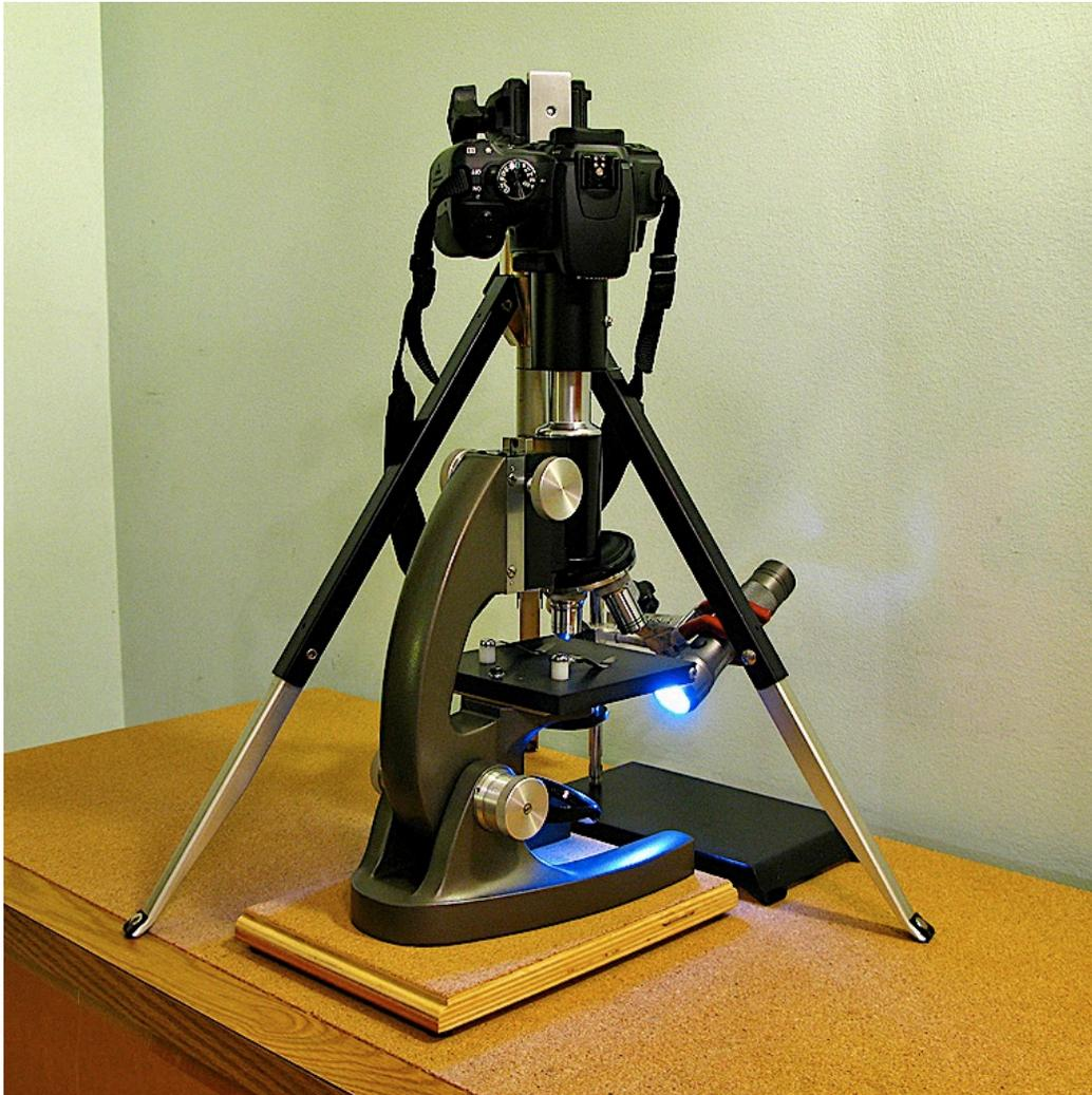
Contrary to what I have read elsewhere, I use an ordinary 10x eyepiece for camera projection, not a specialized photo-eyepiece. As long as the eyepiece is one of the better corrected types, such as a Periplan, Kellner, or achromatic Ramsden, they work fine. A simple Huygens eyepiece, however, produces strong field curvature. I use a Swift 10x widefield.
