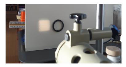
The black ring Blu Tacked into place in each photograph is 35 mm outside 28 mm inside diameter, so similar to the filter holder on many substage condensers.
