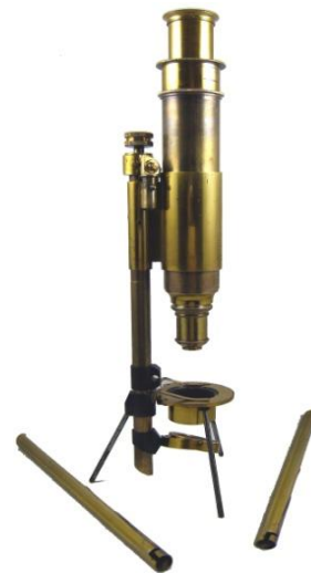
Figure 5. Original Baker Moginie-Style Configured to View Specimens in Liquid
