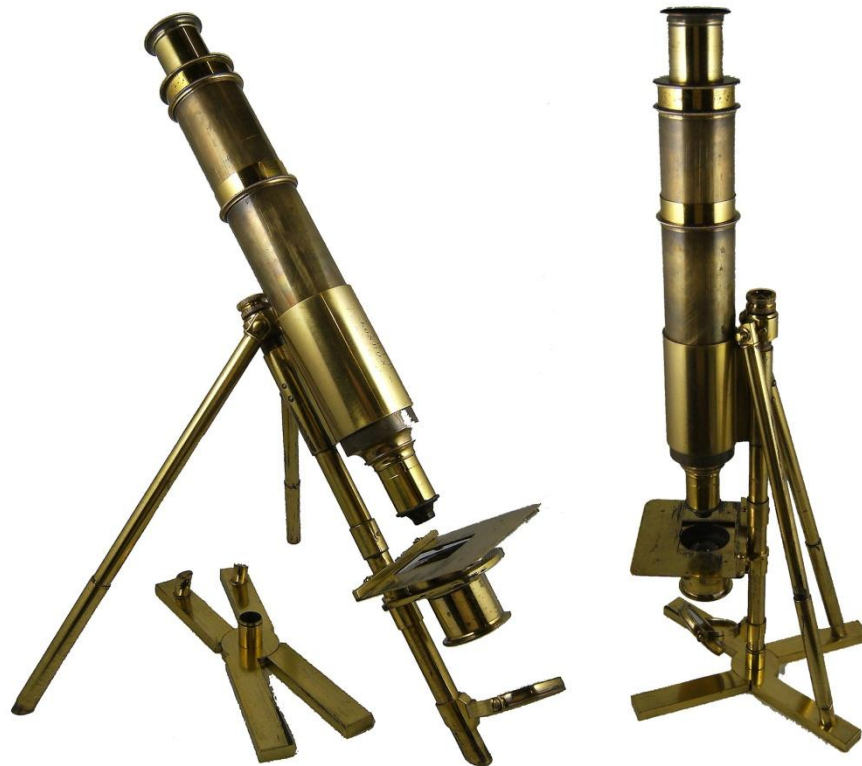
Figure 8. Larger Moginie Showing Cruciform Base Detached and in Use
