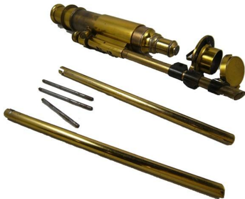
Figure 4. Original Baker Moginie-Style Dissembled Showing Small Legs
