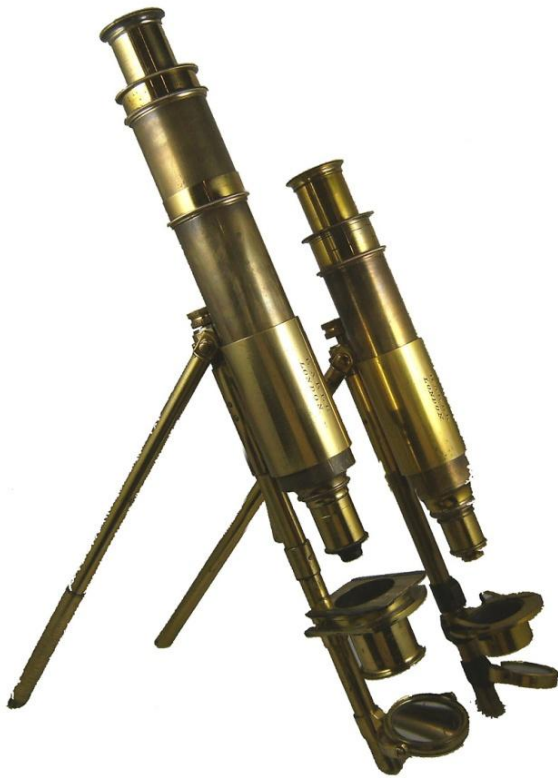
Figure 6. Larger and Smaller Moginies Side-by-Side - Larger With Cruciform Base and Slide-on Stage removed.
