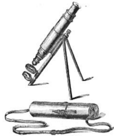
Figure 1. Baker's Traveller's Microscope as shown in Jabez Hogg's The Microscope . 6th Edition (1867)
