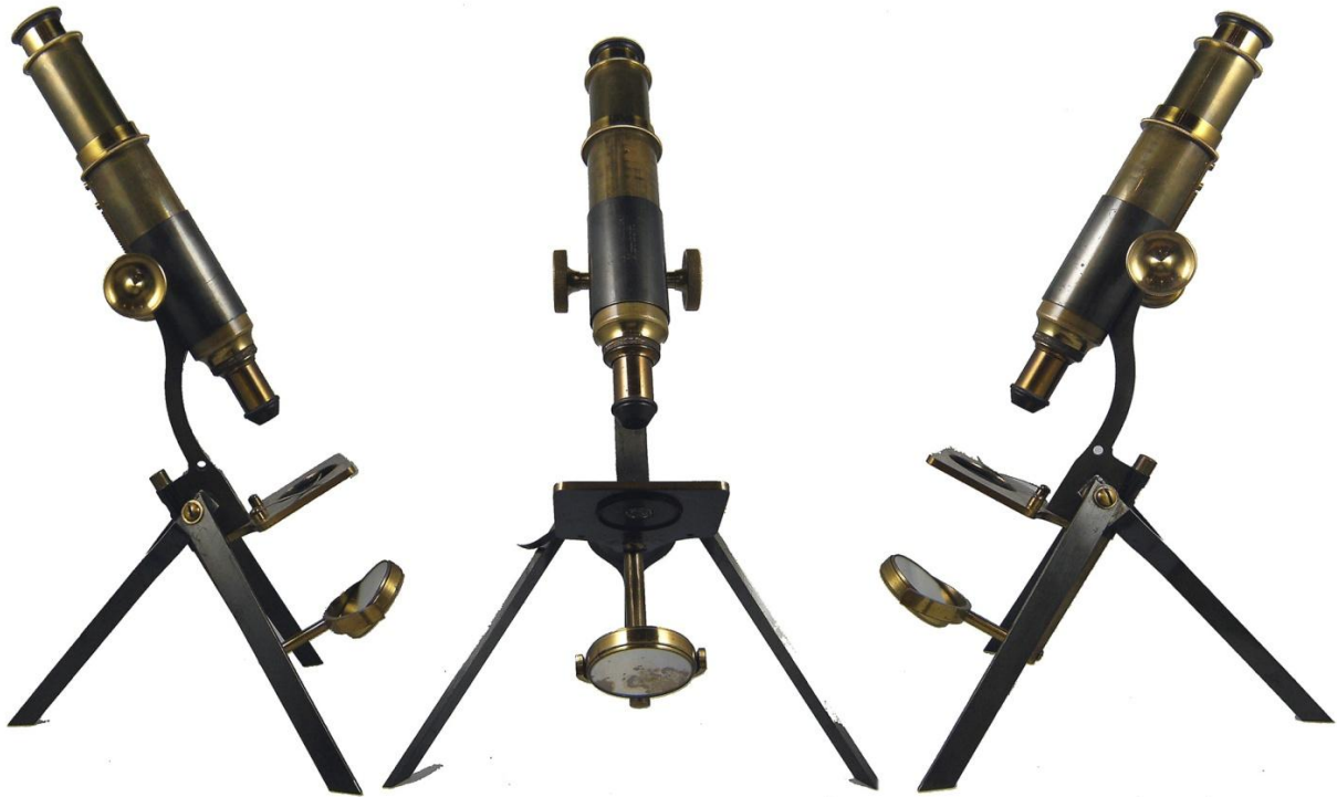
Figure 11. Baker's Folding Field Microscope - A Successor to Baker's Moginie-Style Microscope
