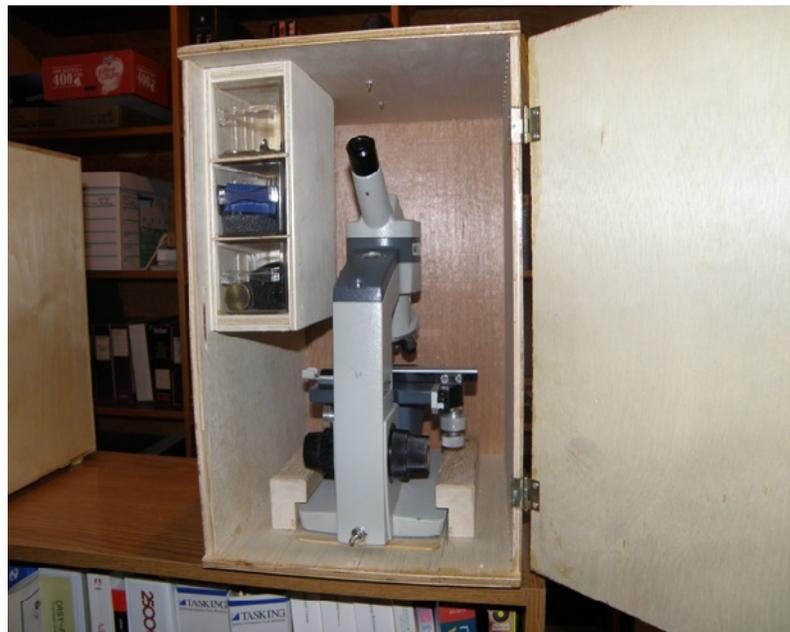
I made a shelf to hold three drawers and on the bottom I fitted some wood blocks to prevent the microscope from moving while in transport. The drawers, I took out of an older parts cabinet. I gave no dimensions or assembly instruction because there is a large variety of microscopes and drawer types. This is just to give ideas on having a traveling lab in one handy case.
