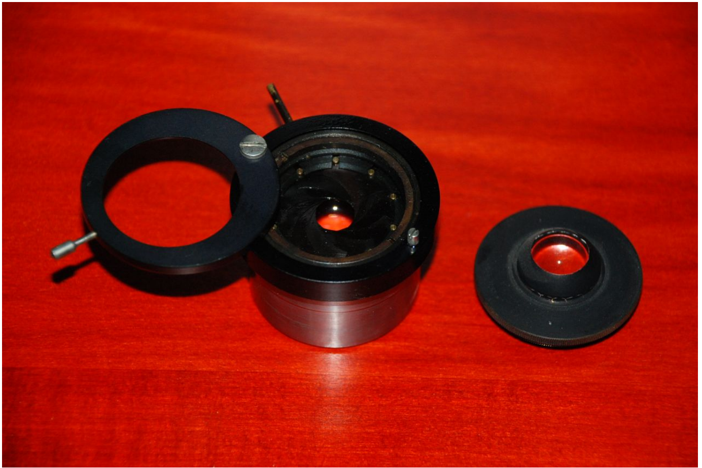
Figure 5. The illumination unit is composed of the filter holder (left), and the iris diaphragm that is attached to the lower side of the condenser. The removable top lens of the condenser is shown to the right.
