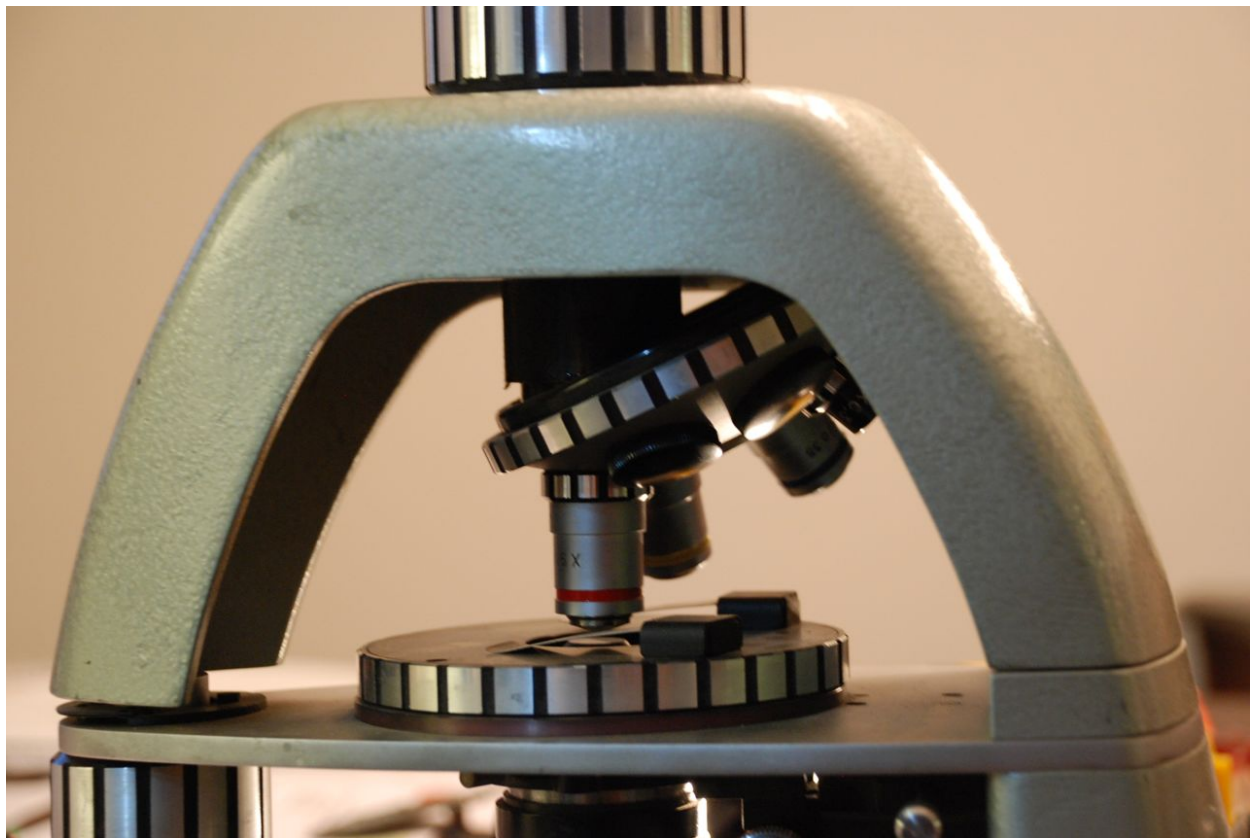
Figure 3. The middle section with the revolving nosepiece, objectives and circular stage.
