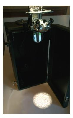
Here are a few samples of projected images. For the most part, there is curvature of field, but the image brightness is commendable.
