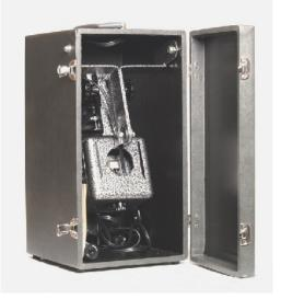
The scope is supported by a yoke bolted to sides of the case. I had to tighten the nuts and bolts severely to be able to position the scope vertically.
