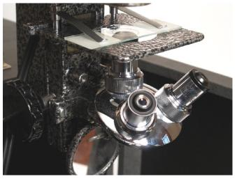
There are two rotating filters between the lamp house and the slide. The first is a heat-absorbing glass filter for use with live specimens such as protists in pond water. The second is a diffusion filter employed when the projection microscope is used as a microscope.
