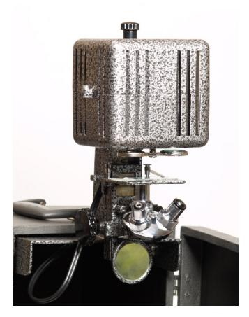
Below the objective turret, there is a first-surface mirror for right angle projection on walls.
