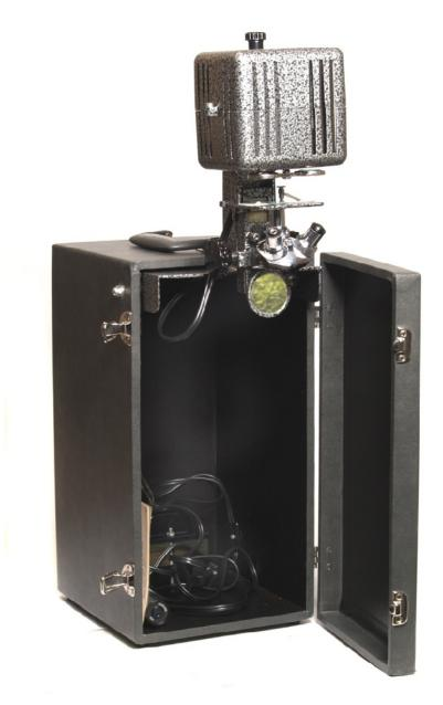
The paint job is an enamel spatter-coating. When I received my copy, the stage clips were on the underside of the stage. I found it was not possible to focus with the stage clips on the underside.
