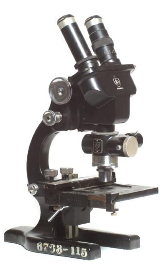
The scope was in remarkably good condition considering it's age at possibly seventy years. The lubricants were not frozen up and the optics free of fungus. Apparently this instrument had been very well cared for. The kit came in an olive drab wooden case, which leads me to suspect this was a "milspec" (military specification) design. The optics were stored in a drawer in the case above the scope.
