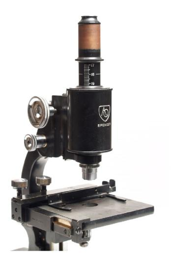
As you can see, the tube length can be varied. The tube does not feature a tube lens.
