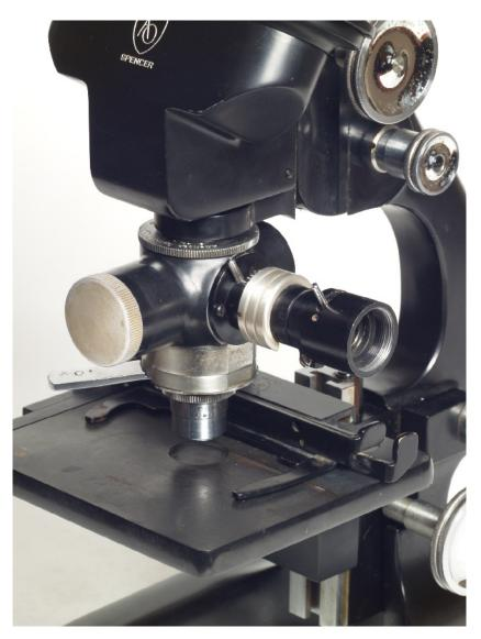
I later found that in order to get a large enough field of illumination using a goose-neck microscope illuminator, I had to remove the field diaphragm to obtain a large enough field of illumination on the subjects.
