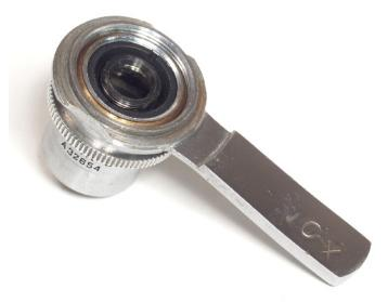
The flange itself has an RMS thread mount, so the objective can be removed to use the monocular tube, which I will discuss later.
