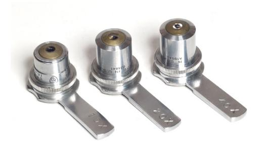
Each objective was mounted in a bayonet flange which fitted the objective into the base of the beam splitter assembly used for epiillumination.
