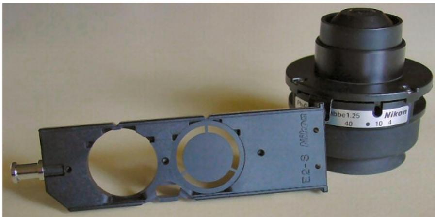
**Figure 6** - The Nikon Abbe slider condenser NA 1.25 oil. The darkfield slider is also depicted.
