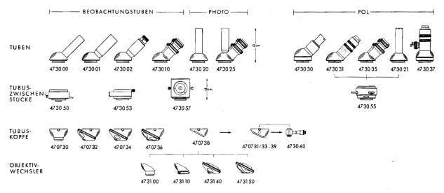
**Legend**: Beobachtungstuben = tubes for observation; Tuben = tubes; Tubuszwischenstücke = intermediate tubes; Tubusköpfe = tube heads (magn changer 47 30 60 last in line, with a tube head with dovetail for interchangeable nosepieces); Objektivwechsler = objective changers for tube head with dovetail.
