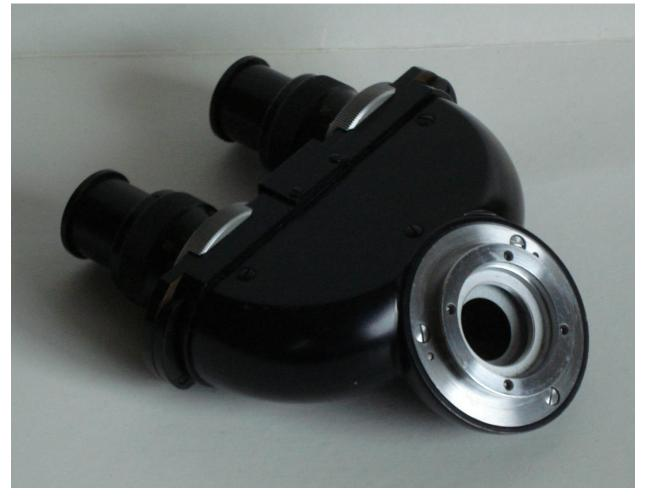
You can see that there is ample space within the circular dovetail to allow for free movement of the optics of the magnification c hanger.
