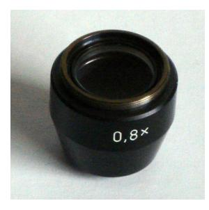
Users of Standard microscopes who wish to have the benefit of this large field can combine the small magnification changer 0.8x shown on page 3 or screw this 0.8x reducing system into their binocular tube which has, conveniently a 28x0.5 metric thread within the dovetail (compare the illustration of the binocular tube on page 2), or, as mentioned already, acquire the special Optovar
