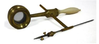
Descendants of the compass microscope were quite popular because of their size and relatively low cost. They were typically unsigned and available in both folding models with turned ivory or wood handles and were typically housed in an étui (Fig. 5) and fixed, non-folding, versions (Fig. 6) which was even less expensive to produce.
