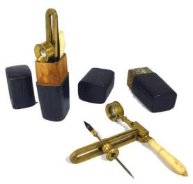
Figure 5. Folding versions descended from the original compass microscopes
