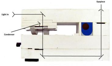
Figure 15. OU McArthur microscope optical path
