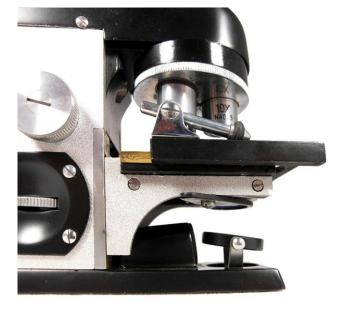
Figure 25. Stage slid outward, away from the microscope
