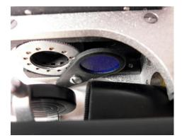
Figure 26. Substage blue filter
