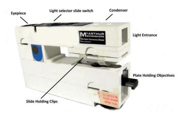
**Optical Heritage.** The optical design of the TWX-1 (Fig. 16) derives from the folded-optics microscopes of John McArthur. But there are important optical differences. To compare these differences the TWX-1 is contrasted here with the ubiquitous Open University (OU) McArthur microscope. This microscope is
