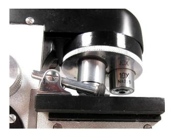
Figure 23. Knurled wheel of triple turret, stage slid inward
