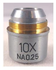
Figure 20. TWX-1 unmounted 10X objective
