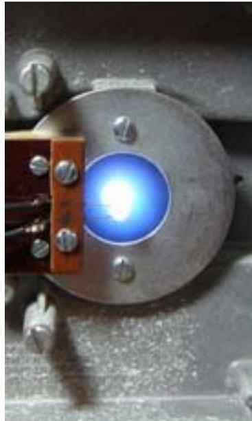
I just clamped the LED leads between two pieces of plastic and bent the leads so that the LED would point towards the bottom of the condenser. At 10mA the LED was bright enough even up to 400X. I wanted to be able to vary the current between 10mA and 30 mA. After some testing I came up with this circuit:
