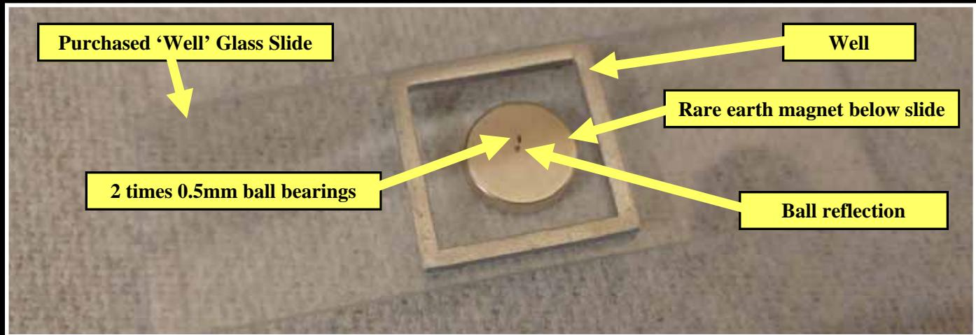
I used a very strong rare-earth magnet to hold the ball in the centre. I moved the ball/balls to one side and put the ,merest hint of UV curing epoxy resin on the slide and moved the balls back onto the resin.
