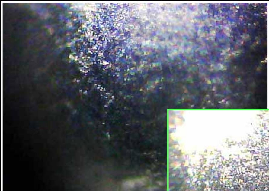
These two pictures were taken at 400x. They clearly show the ball is too rough and granular to reflect an image. The addition issue, is because of the narrow depth of field at increased magnification, the spherical
