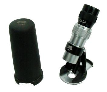
Figure 4. Hensoldt "Tami" inspection microscope
