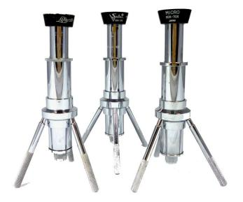
Figure 9. Tripod microscopes inspired by the Spindler and Hoyer "Junior"
