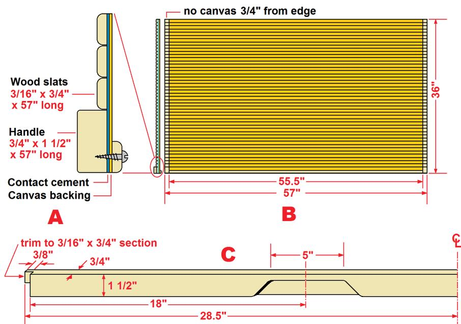
**Figure 4.** Tambour construction. **A:** Detail of construction. **B:** Overview of tambour curtain seen from the back. **C:** One half of the tambour handle; the other half is a mirror image.
