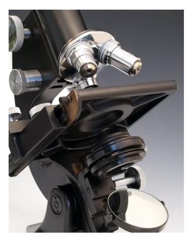
The underside of the condenser has a slot to accept 32mm glass filters or darkfield stops such as my home made ones.
