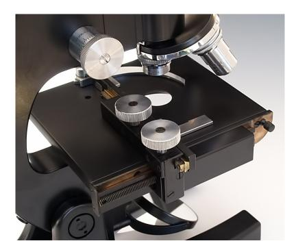
The fine focus knob is graduated in .002mm increments.
