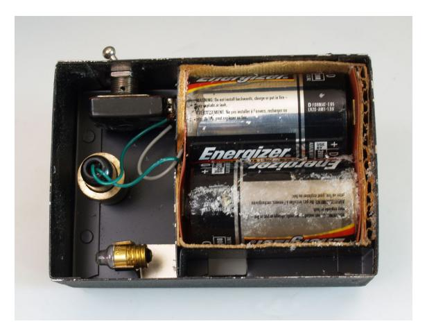
On the right side there is a corrugated cardboard shim to insulate the contacts of the D-battery holder from the chassis of the microscope. Interestingly, the cardboard was scrap from a Japanese battery package for D-cells.
