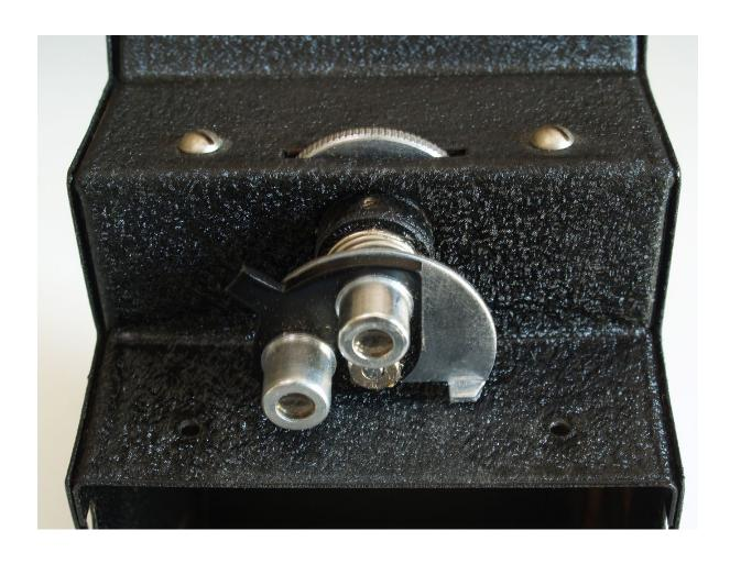
The objectives are rotated with a lever. Just below the stage and above the lamp is a symmetrical doubleconvex lens which serves as a condenser.
