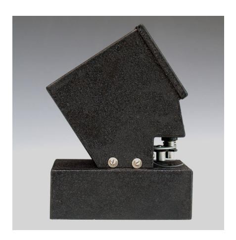
The electronics of the illuminator are fairly basic. In my restoration I replaced the tungsten bulb with a 28,000mcd white LED. I burnished the oxidation from the battery contacts with a Dremel electric motor tool.
