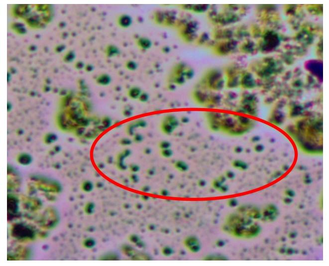
Why cannot we go "further" if we are augmenting the magnification? So-called 'empty magnification' is a factor. Remember that in optical microscopy the limit of observation is given by the light wavelength.
