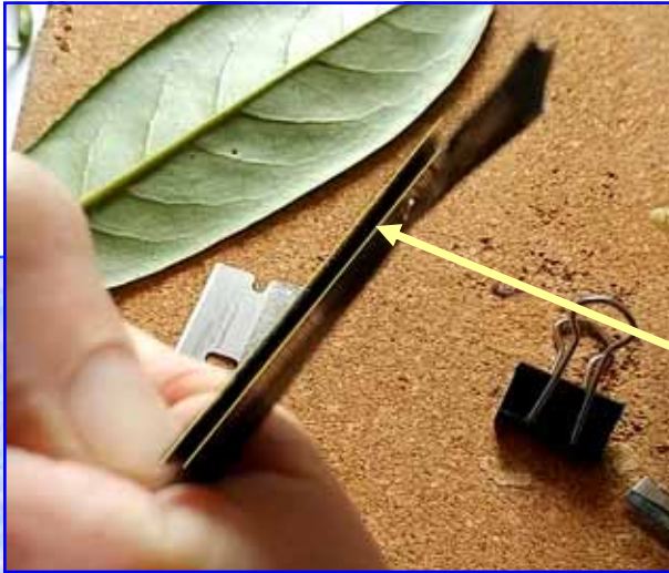
Above: the tape stuck together and the gap left for the cutting edge to poke out.
