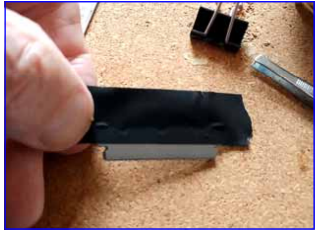
Above: the tape stuck together and the gap left for the cutting edge to poke out.
