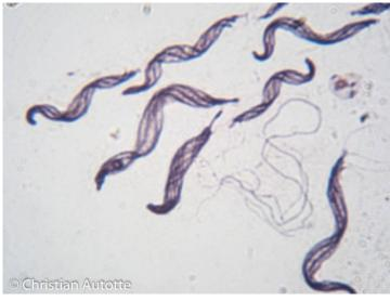
With the 100x lens magnification now reaches 1000x, but without the use of immersion oil resolution is not very good and the image looks blurry.
