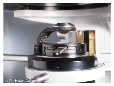
This is the tedious part of working at 1000x; it does slow down the proceedings, but it is a necessary evil. The other part that is very important will be to clean all the oil, especially from the optical surfaces. Lens paper is usually the way to do it, and it must be done quickly once the observing session is completed otherwise the oil may dry up and be almost impossible to clean without the use of xylene or other chemical agent that could potentially be damaging to the optics.
