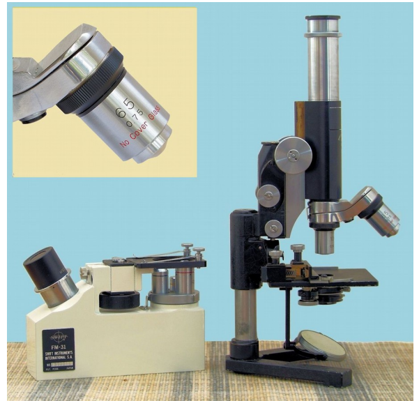
Figure 3. A 1944 Tiyoda MKH and a 1981 Swift FM-31. The MKH is larger and heavier, but is easier and more comfortable to use. It accepts interchangeable optics like this “no cover” objective that is a mainstay of the author’s field work – just one example of a lens not available for folded-light-path designs.
