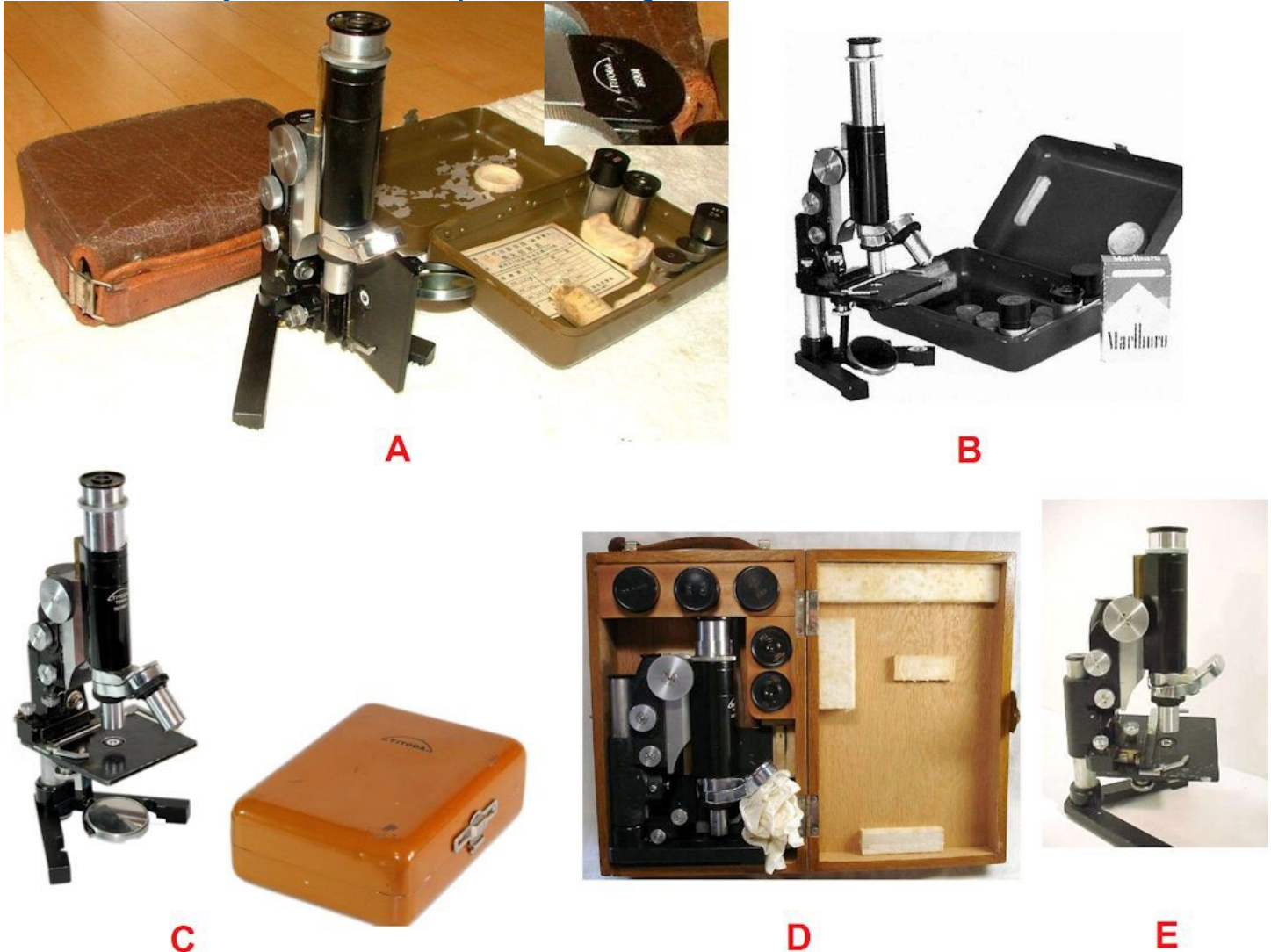
Figure 11. Anomalous combinations of mixed parts: late-war and early post-war mash-ups. A. Microscope with no serial number and with mis-matched cases (April 2014 eBay auction photo.) B. Tiyoda post-war factory image illustrates a microscope without logo or serial number on the tube (History of Tiyoda Microscopes website). C. Third Version microscope serial 14611 with a Second Version foot and Second Version case (Facebook "Portable Microscopes" page). D. A post-WW-II MKH in a wooden case, serial 25392 (March 2011 eBay auction photo.) E. "Kyowa portable" illustrated by Jay Stanley (2006) is probably a Tiyoda unmarked frame with Kyowa-branded lenses attached.
