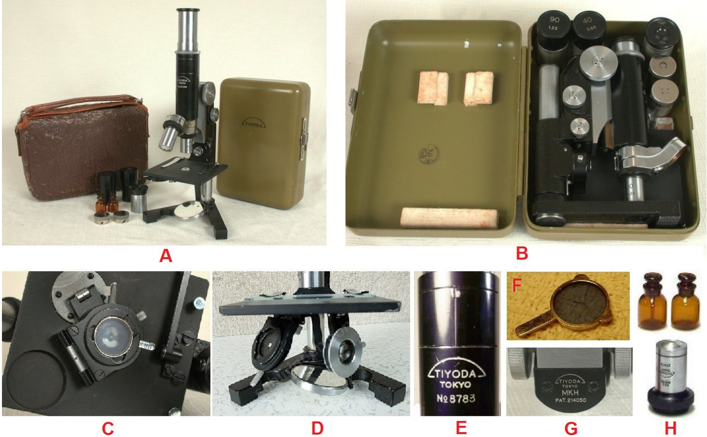
Figure 7. Second Version MKH, produced intermittently from approximately 1934 to 1942. A. Outer soft case and inner hard case. B. Microscope in its hard case. The inspection stamp in the lid has a Showa Imperial date of 17-4 (April 1942). C. Substage condenser is the same as the Heimdal. The stage lock lever is gone; this function was moved to the side of the scope. D. Plain stage with clips. Condenser and iris diaphragm are hanging down for the benefit of this photo; they are not normally left in this position. E. Tube inscription. F. Blue filter in bayonet housing. G. Inscription on the top of the arm. H. 90x immersion lens with immersion oil and solvent bottles. Source of images: A, C, G: May 2009 eBay auction photos of No. 9299. B, E, F: July 2010 eBay auction photos of No. 8783. D: May 2014 photo on Turkish auction site Sahibinden of No. 9329. H: Leitzmuseum.org images of No. 8747.
