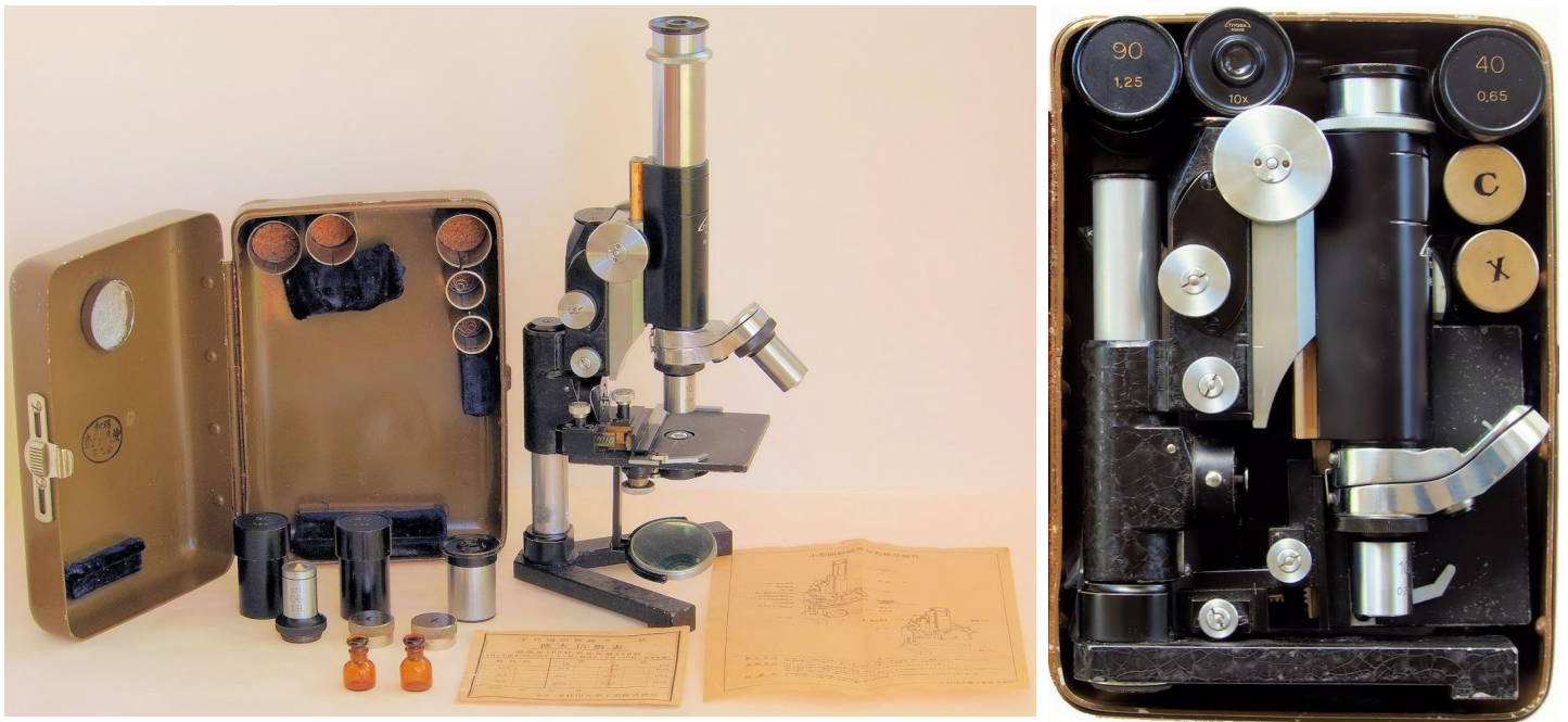
Figure 2. The MKH microscope kit is remarkably compact and portable for a nearly full-size instrument. Tiyoda employees nicknamed it the “Bento” for the similarity of the highly organized storage case to a Japanese bento lunchbox (“History of Tiyoda Microscopes” website). The instruction sheet lists (in Japanese) the kit components: 5x eyepiece, 10x eyepiece, 10x objective lens, 40x objective lens, 90x oil immersion objective lens, cedar oil bottle, xylene bottle, blue glass filter. The inspection stamp in the lid has a Showa Imperial date of Year 19 (1944). This Third Version MKH (author’s scope) is shown in its original configuration; it lacks only the original blue filter and an outer canvas case. The kit in its hard case is 5.1 x 7 x 2.5 inches (130 x 180 x 63 mm). The kit with a substitute outer soft case, four additional lenses, neutral density filters, and polarization filters weighs 5 pounds (2.27 kg).
