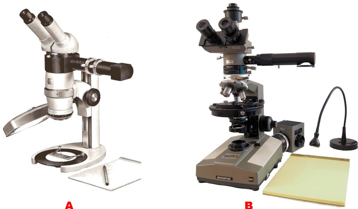
**Figure 1.** Drawing attachments. **A.** On a 1971 Zeiss Stereomicroscope IV (Zeiss catalog image). **B.** On a 1978 Olympus BHAP polarizing microscope (author's microscope). These examples are older models, but drawing attachments are also available for newer and current model microscopes.
