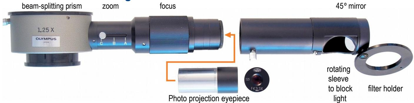
**Figure 2.** Components of the Olympus BH-DA drawing attachment for BH and CH series microscopes.
